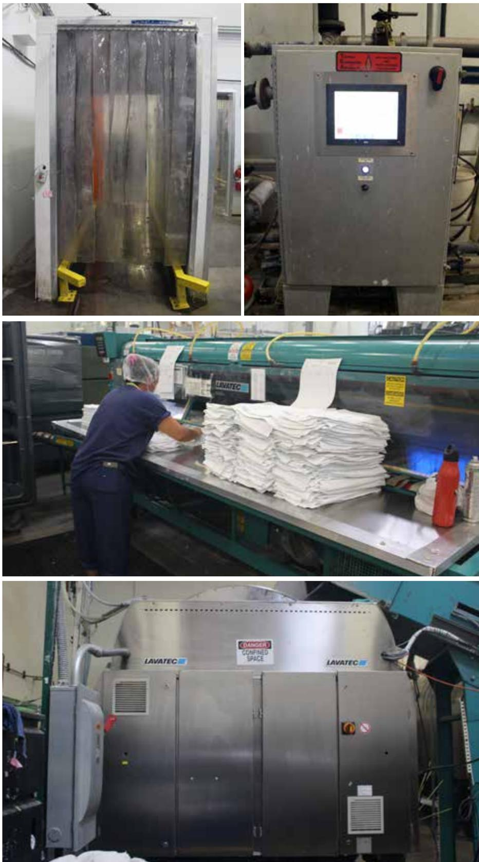
**ABOVE:** (Clockwise, from top) a cart washer; heat-reclamation equipment; an employee inspects stacks of textiles on the back end of an ironing line. One of two tunnel washers in the plant. Sorted goods move up the conveyor at right and drop into the tunnel for processing.
